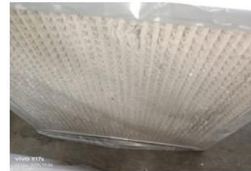
Medium Box Filter single header efisiensi 90-95 %
